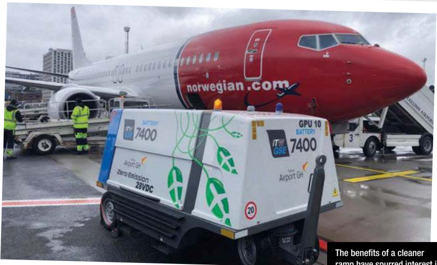
The benefits of a cleaner ramp have spurred interest in ITW's electric GPU solution
