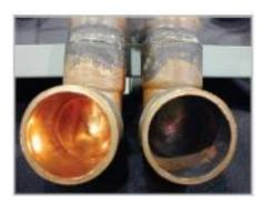
formation can reduce the lifetime of the drier filter and compressor oil significantly. The photo to the right shows examples of tubes, where purge gas was used correct and incorrect.
